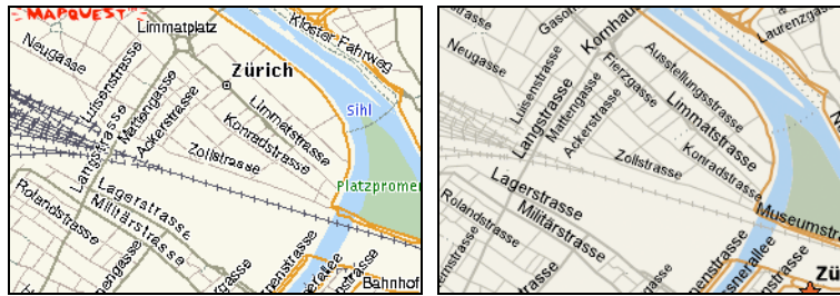
Fig. 2. Web map without (left) and with anti-aliasing (right). Source: MapQuest in the years 2000 and 2006.
