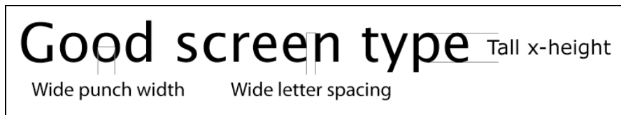
Fig. 11. Good screen type has a tall x-height and a wide punch width.
