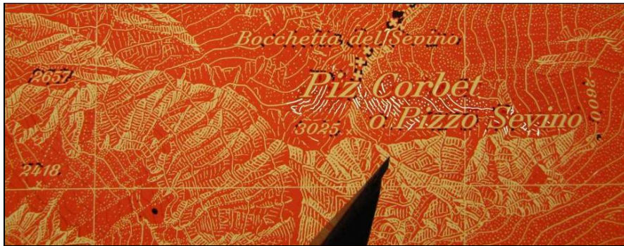
Fig. 1 The rock representation scribed in an etched, red engraving coat with blueprints on a glass plate. The rock scribing tool, a triangularly shaped, whetted steel engraving needle in a wooden holder, is visible in the centre. The pale yellowish map content is etched whereas the bright white shining elements in the centre have been scribed. Enlarged extract from the swisstopo map 1274 Mesocco, 1:25,000, 1998
