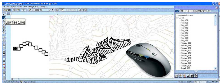
Fig. 3 The rock representation updated with LorikCartographer, enlarged extract from the swisstopo map 1284 Monthey, 1:25,000, 2000. The drawing tool is the mouse
