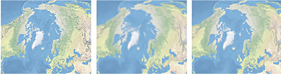
Figure 5. Texture sampling: noisy bilinear sampling (left), trilinear mipmap sampling, blurred around poles (center), and trilinear mipmap sampling with anisotropic filtering (right). Screen captures are enlarged for visualizing graphical artifacts.
